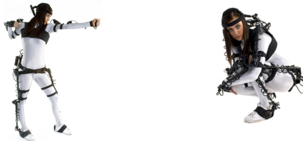
Figure 2.1: Gypsy 5, by Animazoo, an example of a mechanical motion capture device.
